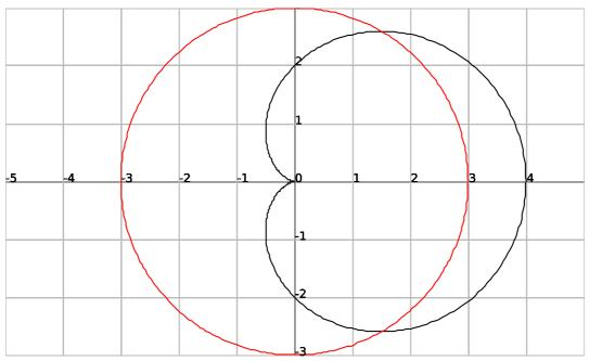
These two polar curves intersect when  $2+2\cos\theta=3\Rightarrow 2\cos\theta=1\Rightarrow \cos\theta=\frac{1}{2}\Rightarrow \theta=-\frac{\pi}{3}$  or  $\theta=\frac{\pi}{3}$ . Using symmetry, we will integrate from  $\theta=0$  to  $\theta=\frac{\pi}{3}$  and double that area.
